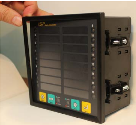
Picture1-Gently hold and unlock front panel frame at one side as shown
